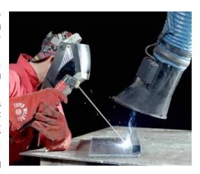
Regardless of duration, HSE will no longer accept any welding undertaken without suitable control measures in place, with these new stipulations also applying to welding outdoors. Risk assessments and safe systems of work should be updated to reflect the change, RPE should be subject to a suitable programme of checks and LEV systems should be thoroughly examined by a competent person and tested annually.
